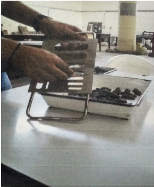
Fig. 1 Metal gauge for flakiness index
